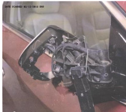
Image 5: severely damaged passenger side mirror
