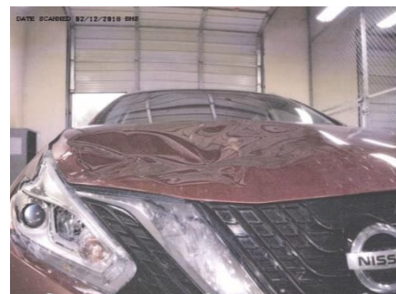
Image 7: damaged right side hood and grill
